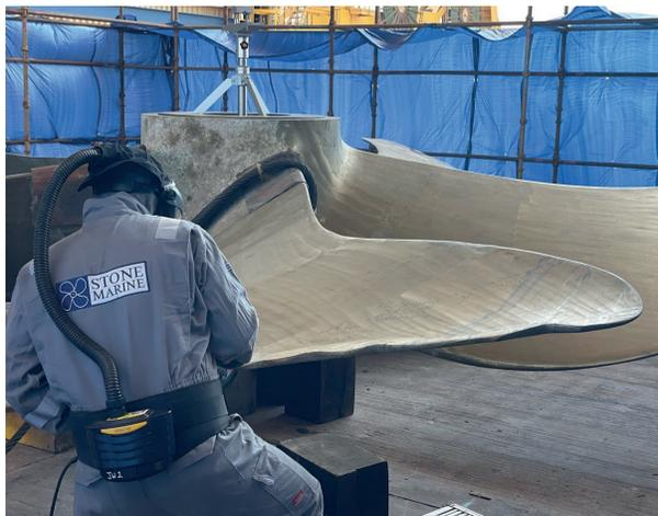
A STONE MARINE SHIPCARE TECHNICIAN IN ACTION REPAIRING A DAMAGED PROPELLER
